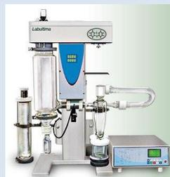
Dissolution Tester and Spray Dryer
